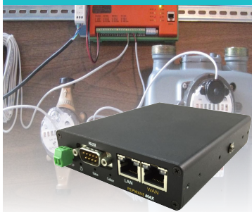
BR1 M2M -RS232 interface. -Optional DIN rail mount.
