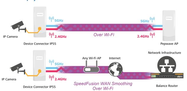
Using the Device Connector IP55, the IP camera is able to upload videos network is using an AP from another vendor, frequency combination can using both the 5GHz and 2.4GHz frequencies at the same time. If one also be achieved by forming a SpeedFusion tunnel between the device frequency loses connectivity, the other will seamlessly take over. If the connector and a SpeedFusion-enabled router.
