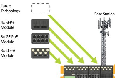
Equipped with an EPX, mobile headquarters can combine private LTE, commercial LTE and satellite links to form a fast, unbreakable VPN connection to headquarters and to patrol vehicles. With this configuration, patrol vehicles benefit from
