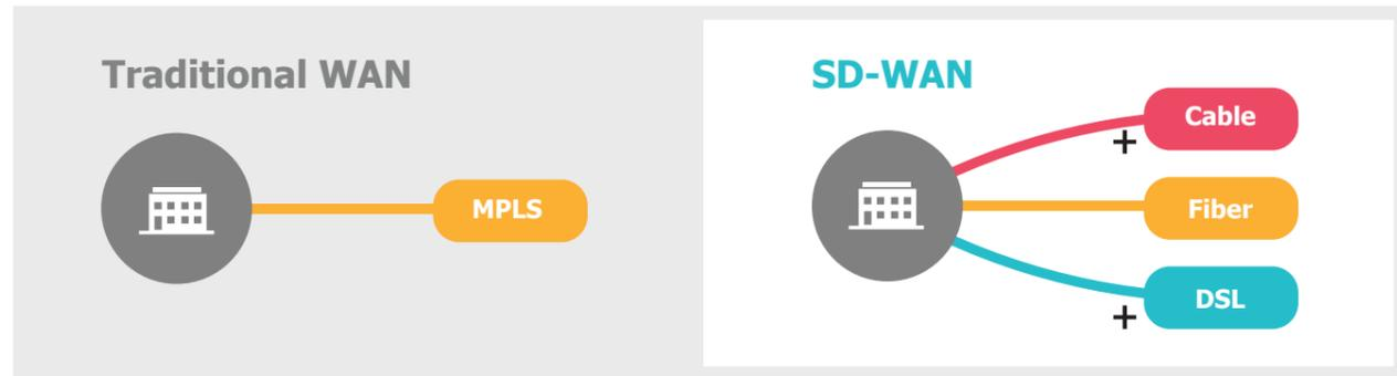
**Greater Flexibility:** Peplink routers are capable of taking multiple Internet links and turning them into a single connection. To increase speed or reliability, simply add more links.
